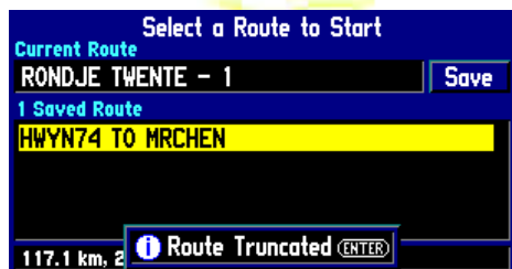
(fig. 4) Route split up. This means that the route is in fact simply cut off at that point. Bottom left is shown at what distance that happens.
